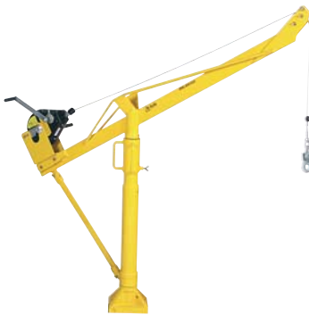
Davit Arm and Bollard BCS0010, BCS0014, Base BCS0012 – for entry to confined spaces, 600kg rated, 1200mm reach, 1800mm lift height.
