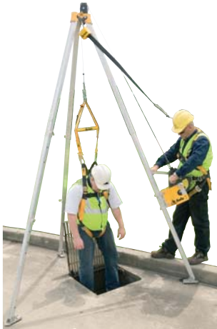
BR02001K Tripod – 2.2m to 3m height, fully adjustable legs, alloy construction, spring locking leg pins, pulley wheel in head, rated to 200kg.
