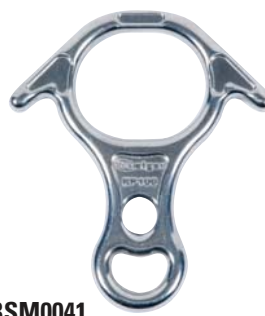
BSM0041 Rescue figure of 8 9 – 13mm rope 35kN
